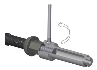
Turn the screw part of the adapter by using the integrated lever. Now the adapter is firmly and tightly connected with the injection nut of the RG bolt and ready for grouting. The sealing guarantees that no grout sprinkles out.
