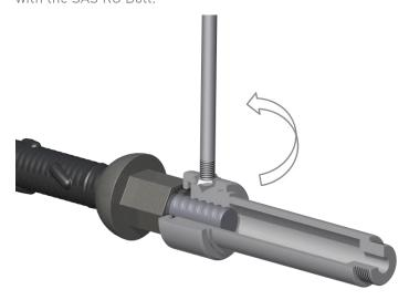
Turn the screw part of the adapter by using the integrated lever. Now the adapter is firmly and tightly connected with the injection nut of the RG bolt and ready for grouting.
