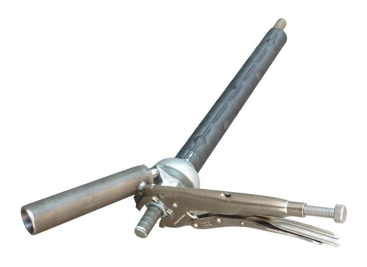
The injection nozzle is welded on a pliers. After inserting the nozzle into the injection channel the pliers is pressed and thereby the nozzle is fixed in the channel. The grouting process can be started.
