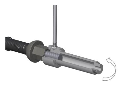
Screw the injection adapter above the SAS thread bar shortly before the injection nut. The position of the inner thread of the adapter has to be above the flat side of SAS thread bar.
