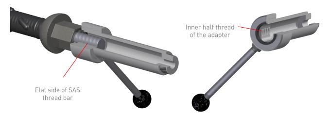
Push the injection adapter above the SAS thread bar shortly before the injection nut. The position of the inner thread of the adapter has to be above the flat side of SAS thread bar.
