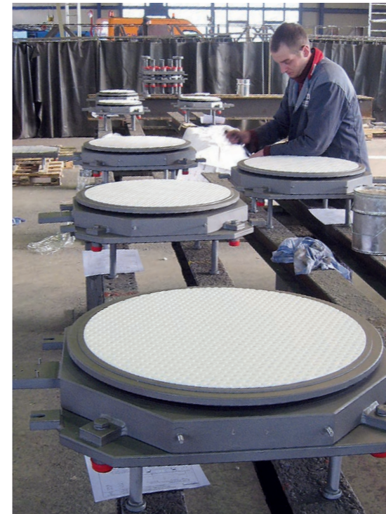
Assembly of free sliding pot bearings
