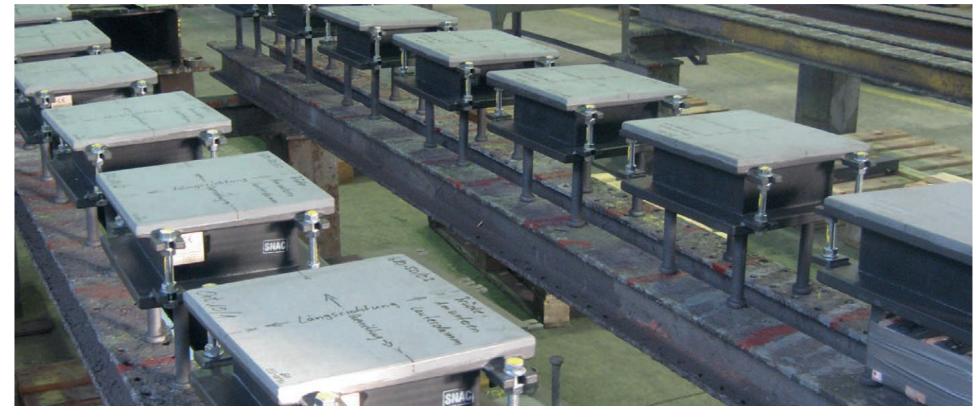
Final assembly of elastomeric bearings in the SCHREIBER plant
